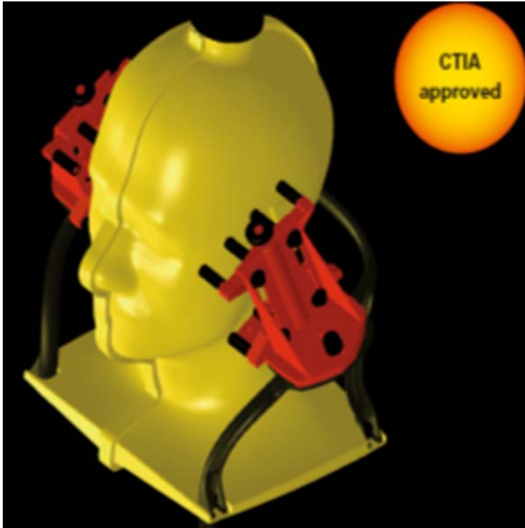
FIGURE 1 SAM Phantom. Source: Speag Phantom Product Flyer. “CTIA” is Cellular Telecommunications Industry Association.
